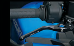
Billet brake lever (Anodised) Machined from high-end billet aluminium and decorated with the GSX-S logo, these black anodised levers enhance the bike's sporty good looks.
